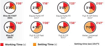
Setting time (sec) 23±1°C Source: Internal test data Nov 2020 \*Not a registered trademark of SDI.
